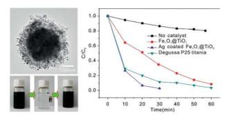
Ag-coated Fe<sub>3</sub>O<sub>4</sub>@TiO<sub>2</sub> microspheres with a very good core/shell structure, show excellent magnetic properties at room temperature. The formation of a Ag-TiO<sub>2</sub> heterojunction results in good photodegradation properties of the products. The results show that the as-prepared composites can be used as convenient and recyclable photocatalysts.
